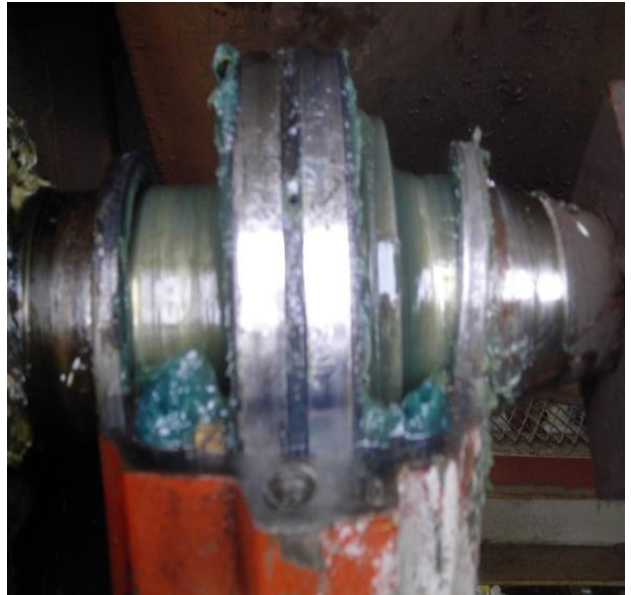
The bearing shows no evidence of contamination
