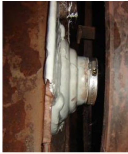
Bearing shaft and bearing drum for the conveyor belt after applying Oxifree
