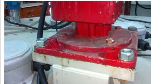
Oxifree coating peeled off from the nuts on the front of the agitator. Stainless steel nuts still shiny compared to corroded nut at the back of the agitator.
