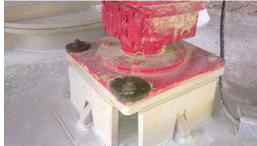
Oxifree coating after exposure to operating environment for 10 months. This tank and agitator is more exposed to the outside environment and is also exposed to lime and neutralisation products.
