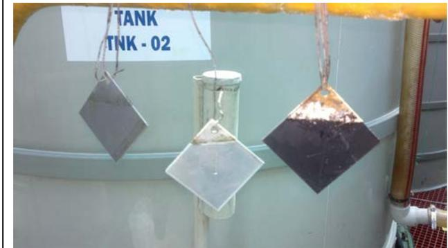
From left to right: stainless steel, aluminium and mild steel with the Oxifree coating removed.
