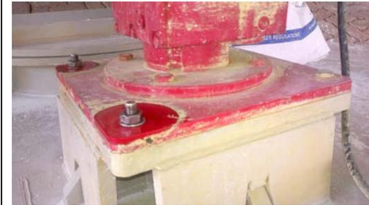
Oxifree coating peeled off from the nuts on the left of the agitator. Stainless steel nuts still shiny compared to corroded nut on the right of the agitator.
