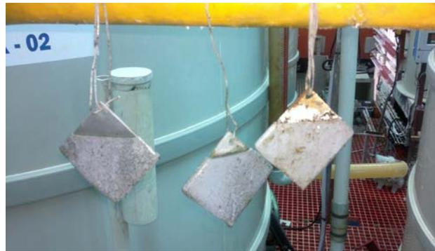
From left to right: stainless steel, aluminium and mild steel with the Oxifree coating in place.
